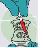
Press the plunger of the Minivette®. Make sure you hold onto the cartridge while doing this so that you don't knock it over and spill the contents.
